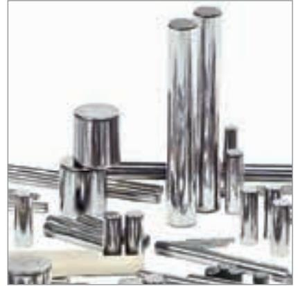
The profile of the lateral surface of this kind of rollers - type ZB - is composed of the cylindrical middle section and the slightly laterally chamfered end zones. This type of end profiling prevents harmful stresses to the edges. Cylindrical rollers are suitable in different applications, mainly:
